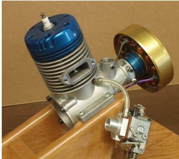
Temporarily install alternator
