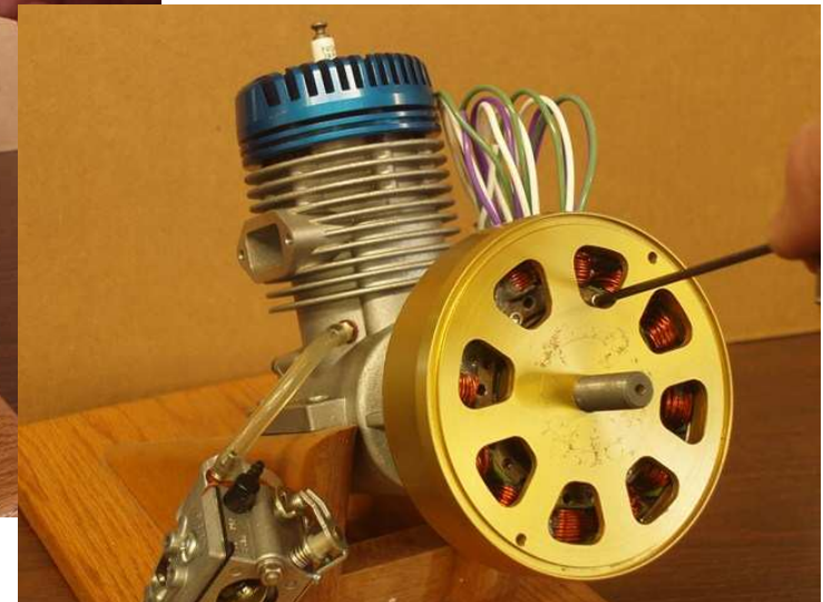
Install and tighten all stator bolts
