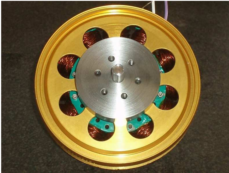
Remove fixtures, rotor may need to be turned to Access all screw heads
