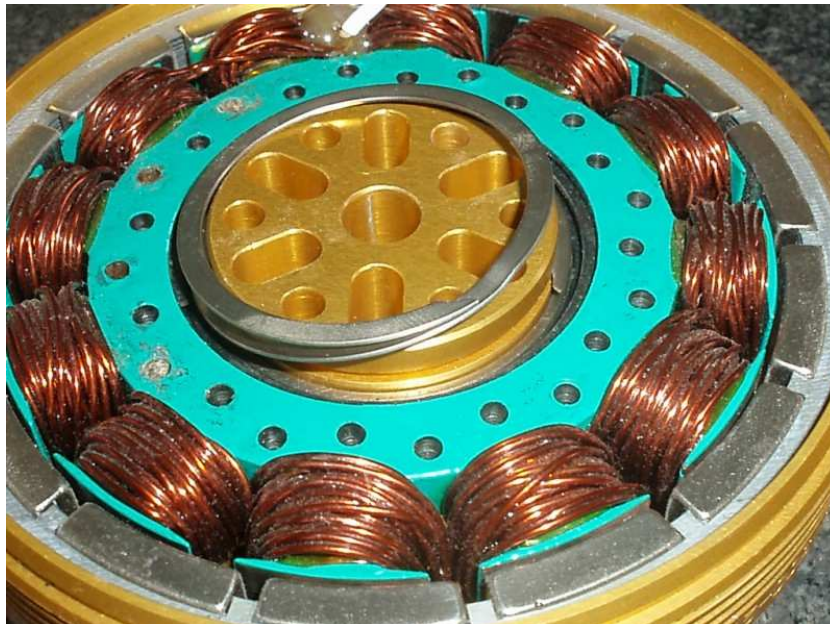
Install retaining ring in groove in rotor hub
