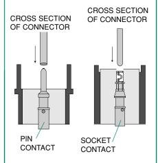
4. Carefully remove the extraction tool from the connector to avoid damage to the insulator.
