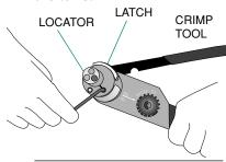
3. Select the proper locator position for your contact by rotating the locator until the proper color is aligned with the index mark. Push locator back down until it snaps into position.
