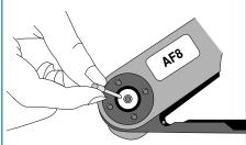
6. Insert the stripped wire into the contact with a slight twisting motion. Be sure all wire strands are inside the contact. Squeeze the handle to cycle the tool. The handle will not release until the contact is completely crimped.
