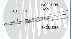
3. Lubricate the grommet with isopropyl alcohol (do not use any lubricant other than isopropyl alcohol). Insert the contact through the appropriate cavity in the grommet. Sizes 16S, 16 and 12 SOCKET contacts must be installed using guide pins. See the Contact Selection Guide on page 103 for Insertion Guide Pin part numbers.
