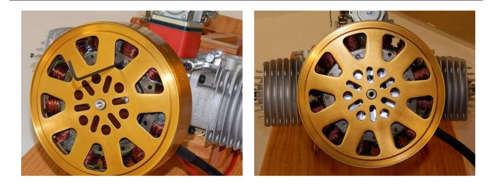
**Step #3:** Using the bolts provided, attach the Stator to the mounting bracket using either lock washers or retaining compound. Once all bolts are in place proceed to the next step.
