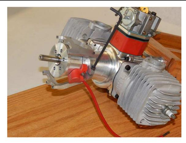
**Step #1:** Remove Prop Bolts and Washer, locate and take note of Hall Effect Sensor, and loosely attach Clamp Style Alternator Bracket with retaining compound and the hardware provided.
